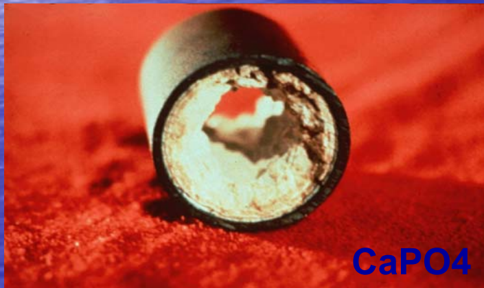
Scaled Heat Exchanger Tubes
